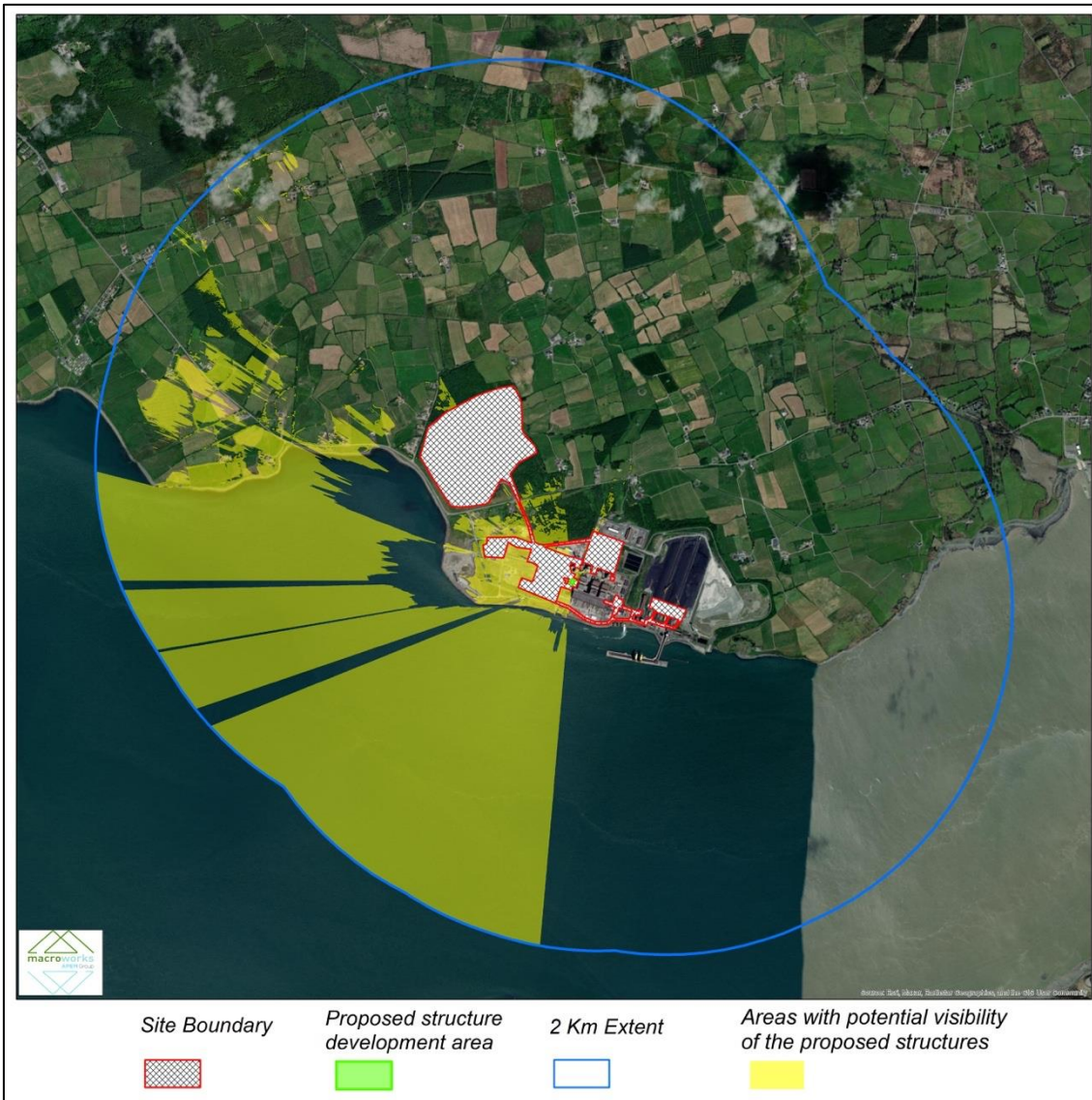
Figure 14.5: ZTV map for the proposed auxiliary boilers based on a Digital Surface Model that accounts for screening by surface elements such as existing buildings, hedgerows and trees lines
