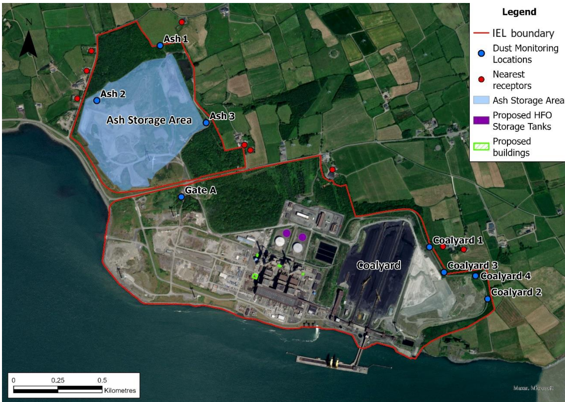
Figure 7.4: Dust monitoring locations and nearest receptors
