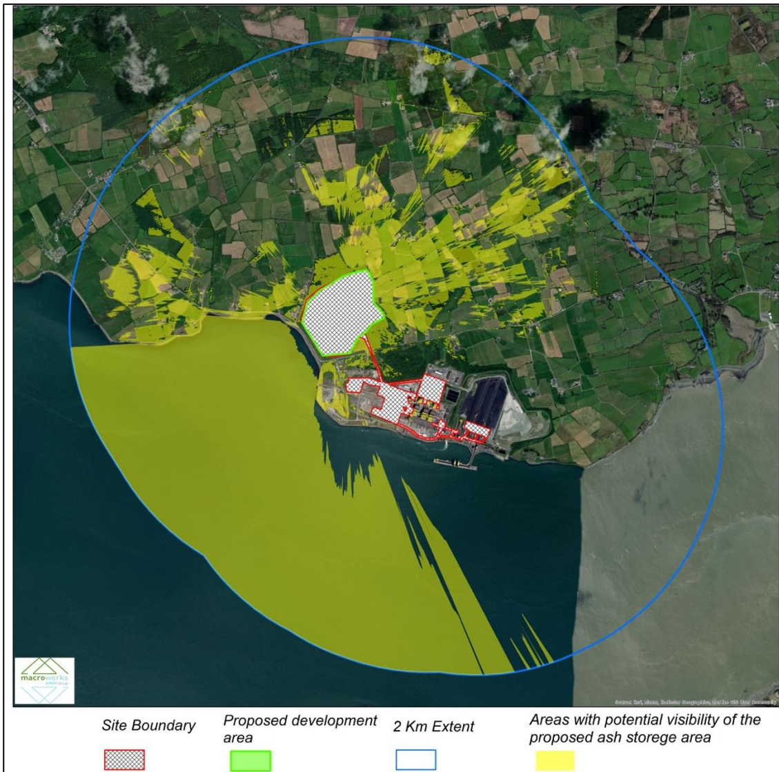
Figure 14.6: ZTV map for the proposed changes to the Ash Storage Area based on a Digital Surface Model that accounts for screening by surface elements such as existing buildings, hedgerows and trees lines.
