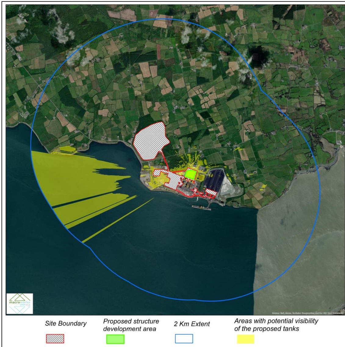
Figure 14.4: ZTV map for the proposed HFO tanks based on a Digital Surface Model that accounts for screening by surface elements such as existing buildings, hedgerows and trees lines.
